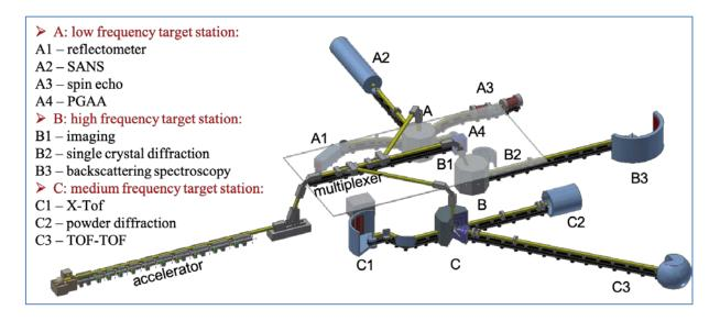
Fig. 3: Possible layout of a High Brilliance Neutron Source HBS. Instrument with the same requirement for pulse time structure are grouped around the same target station. Different target stations with different pulse structure are being deserved by multiplexing the ion beam from the accelerator. Each instrument has its own dedicated moderator /8/.
